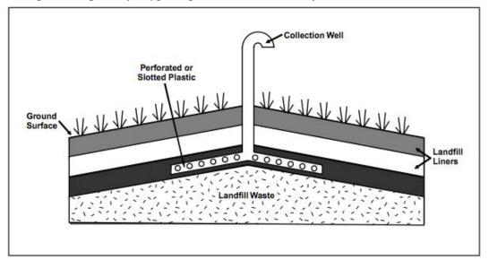
Image 7. Diagram of a typical passive vent in a landfill.
